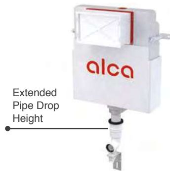
WRAS Alca Concealed Cistern AM112 £204 H 480 x W 510 x Instl. Depth 145-220mm (Size Exc. Pipe Drop)
